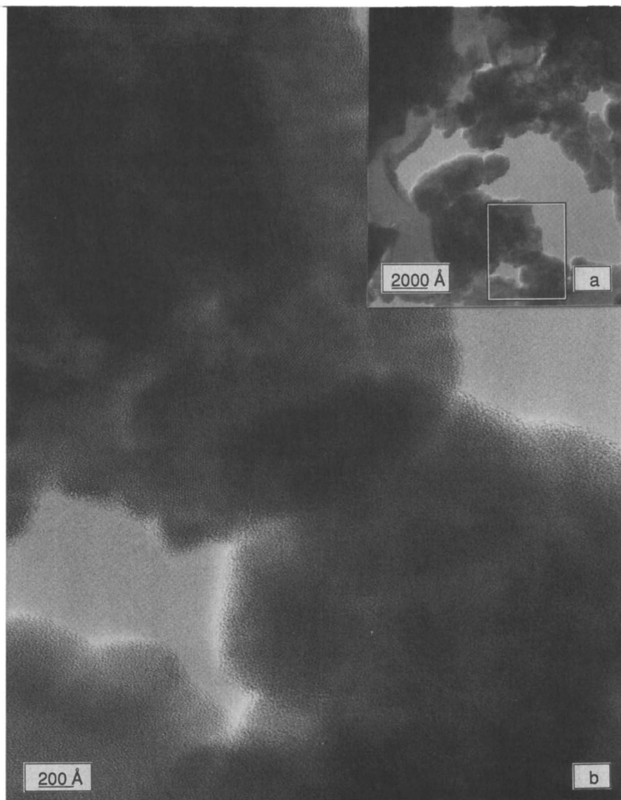
Figure 8. (a) Isolated USY crystallite within Fraction F, and (b) Lattice image of USY crystallite within Fraction F.
